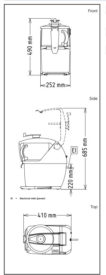
Electric Supply voltage: 200-240 V/1N ph/50/60 Hz Electrical power, max: 1 kW **Total Watts:** 1 kW Capacity: Performance (up to): 550 kg/hour Capacity: 4.5 litres **Key Information:** 252 mm External dimensions, Width:
